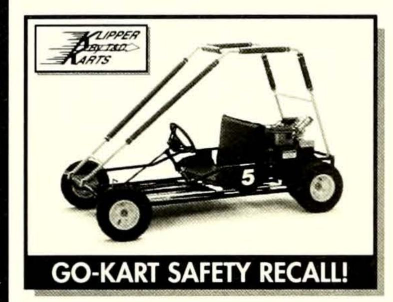
CPSC has determined that long hair and long loose clothing can become entangled in the rear axle of a KLIPPER KART, and misuse can cause bodily injury or death.
