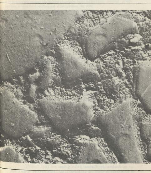
COVER PHOTO. The X7700 electron micrograph appearing on the cover is of a silicate cement after setting. The core is unattacked powder particles surrounded by a silicic acid gel matrix.
