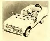
R. New Bronco Roadster has no cab roof or doors and features a windshield which can be folded flat and secured to the hood. A bench seat is standard. (Ford Motor Co.)
