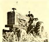
S. New seven-plow 1206 Turbo tractor is designed for high-speed farming. The Turbo engine provides more power with less smoke and noise. (International Harvester Co.)
