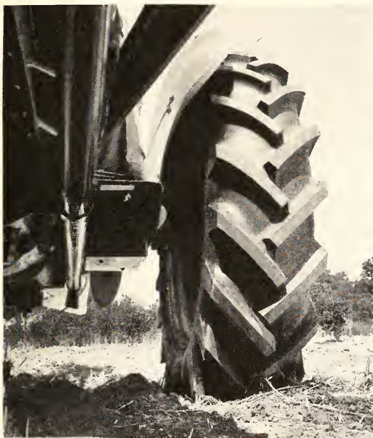
BIGGER CLEATS—BIGGER SHOULDERS on this new B. F. Goodrich Power-Grip tire. Those big cleats are curved to prevent bending. They're broad at the base to give extra rigidity.
