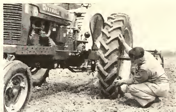
MORE RUBBER—MORE FOR YOUR MONEY. That's what farmers like about the BFG Power-Grip tire. The bigger area on the face of the cleat means more pulling power. And it's a self-cleaning tread.
