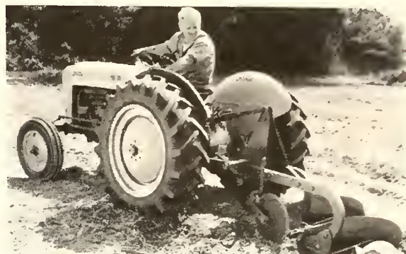
BIGGER CLEATS—BIGGER SHOULDERS on this new B. F. Goodrich Power-Grip tire. Those big cleats are curved to prevent bending. They're broad at the base to give extra rigidity.
