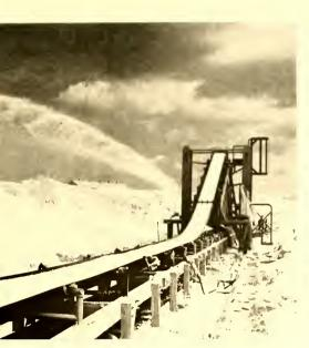
High speed belt slinger places salt in storage piles until needed at the mill.
