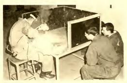
Viewing a welding demonstration through this protective material allows nine students to watch at the same time.
