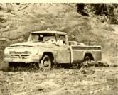
Roll over sand, mud or snow with one of our all-wheel drive models. They're equipped with two speed power-dividing transfer case controlled by a single stick.
