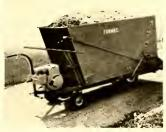
H. New self-powered Mobilfeeder eliminates pushing loaded feed carts and forking feed to cows. (Farmec, Division of New Holland)
