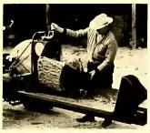
New Bles Easy Woodsplitter is easily attached to power take-off of small tractors to split hardest wood. (Bles Axe Co.)
