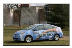
The preliminary data from the road tests of these vehicles indicate that the fuel efficiency of these vehicles is improved by as much as 90 percent within a commuting distance of 40 miles or less. This improvement in fuel efficiency also factors in the energy cost due to recharging of the battery from a power outlet. Since it is expected that a PHEV would recharge during the overnight hours, the load on the power grid occurs during a period of lower overall electricity usage.
