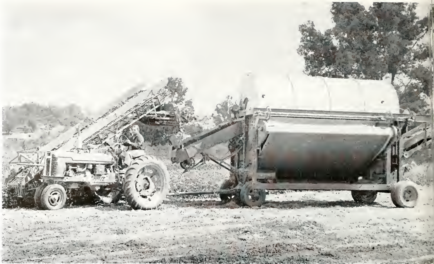
Claude harvests his 88 acres of lima beans with a machine that shells the beans.
