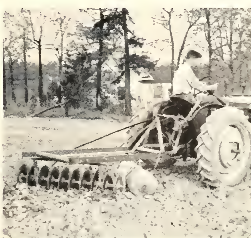
Leon Paulette, above, is showing how his pickup-type disk harrow operates. He made the harrow in his vo-ag shop from old disks and scrap metal.
