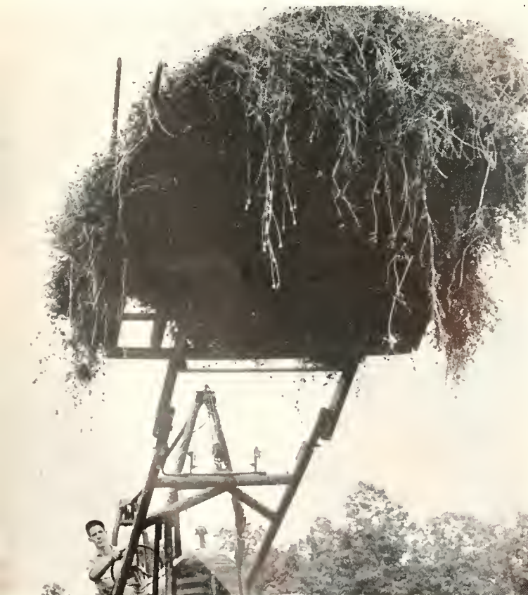
The new power lift operates on any tractor. Here Leon is loading hay with the lift and buck rake attachment.
