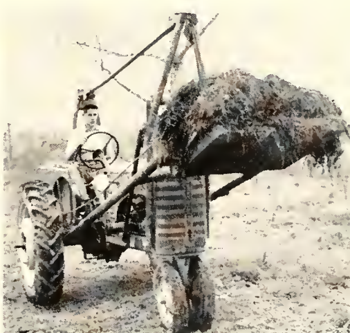
Young Paulette made still further use of the winch by making another labor saver—a tractor-operated manure loader. Here he demonstrates its use.
