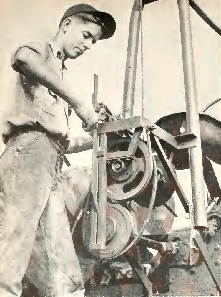
Leon Paulette makes a minor adjustment on his tractor power lift. Its new features earned a U. S. patent.
