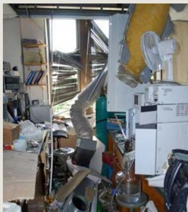
Hydrogen gas has an extremely broad explosive range. The photograph on the left was taken inside of a university laboratory in Missouri after a mixture of hydrogen and nitrogen exploded inside of an incubator. Although the explosion occurred in 2010 it still serves as a
