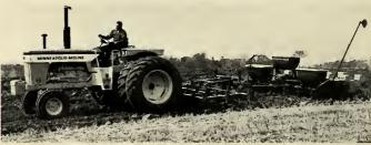
S. New Vista row-crop tractor features high and low range shifting-on-the-go in five forward speed ranges that reduces speed 30 percent and increases torque 46 percent for heavy loads. Also has a transmission oil cooler for more durability. (Minneapolis-Moline)
