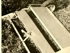
Adjustable flick bar pushes the crop into feeding position, feeds it butt first.
