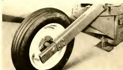
Exclusive adjustable wheel flips over to fit any row-crop spacing.
