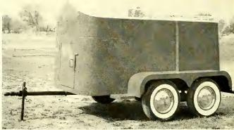
The finished tandem-wheel trailer was made largely from scrap angle iron and sheet metal. It is built low for loading and can haul all sizes of livestock.
