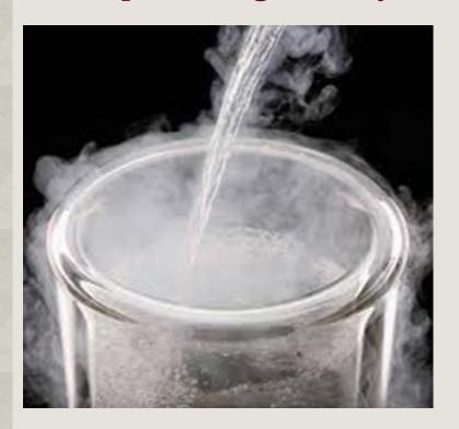
Liquid nitrogen is a common component of research operations, however are you aware of the hazards of cryogenic liquids, such as liquid nitrogen? Do you know the expansion rate of liquid nitrogen? You have probably heard of the potential for liquid nitrogen spills or leaks to produce an oxygen deficient environment, but did you know you could also produce an oxygen rich environment near the liquid nitrogen source?
