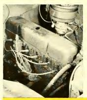
Engine block covered with grease and lost oil filter cap indicate neglect.
