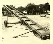
Entire 28-foot bale elevator has been made in vo-ag shop with exception of chain, PTO, and wheels. Galvanized metal conveyor pan was crimped in local sheet metal shop in 10-foot sections. Wheels and spindles are from junk yard; hand-cranked winch is shop-made. Paddles, frame, and hitch come from scraps.
