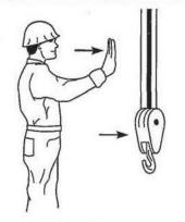
BRIDGE TRAVEL. Arm extended forward, hand open and slightly raised, make pushing motion in direction of travel.
