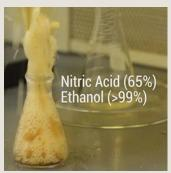
Nitric acid that has been added to waste jugs containing alcohol has caused numerous container to rupture at institutions across the nation because of the pressure build up from the gases released by these incompatible chemicals when mixed together.
